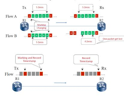
Alternate Marking Method (RFC8321)
